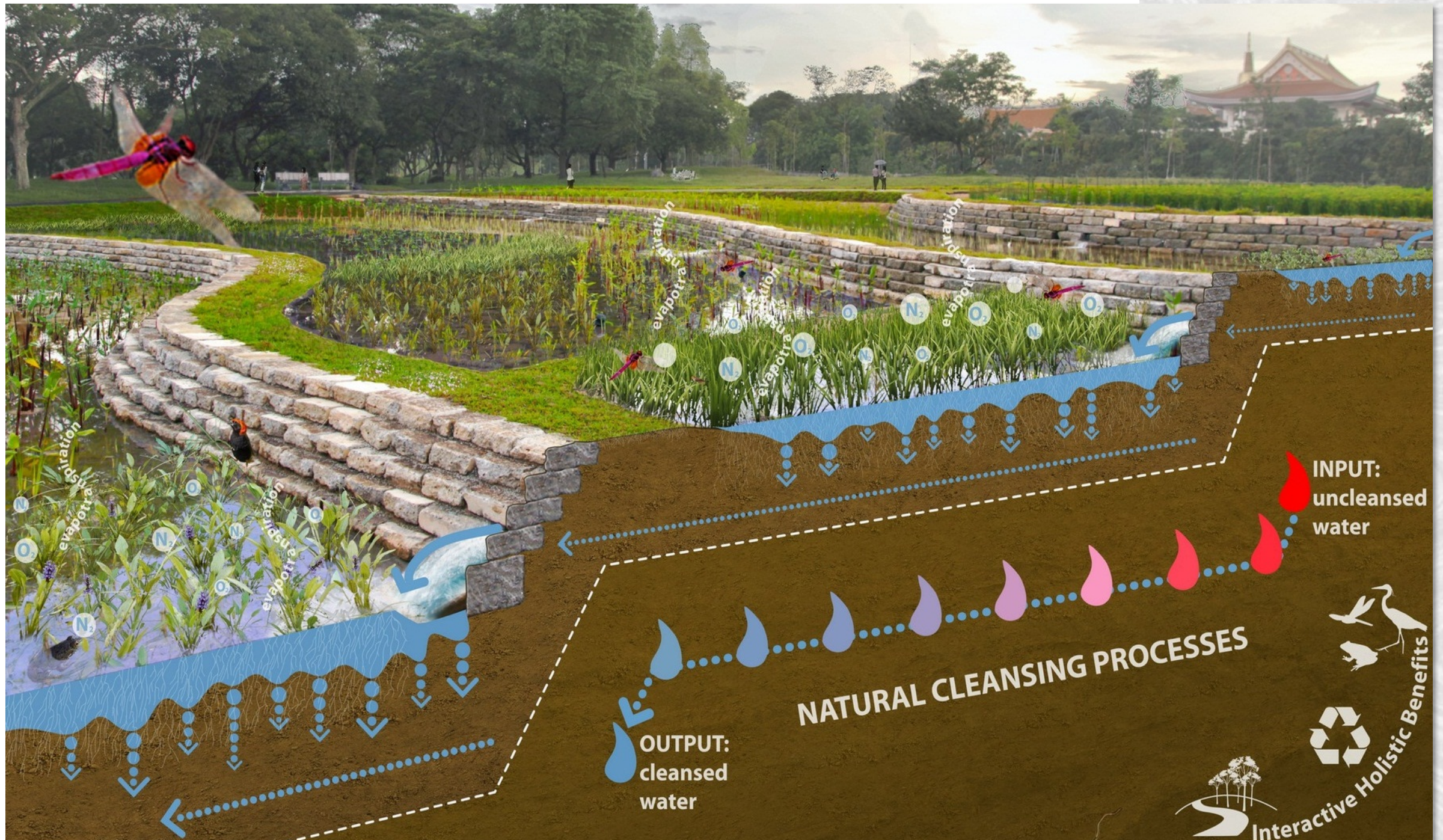
Cleansing Biotope System Schematic: Bishan Ang Mo Kio Park, from Atelier Dreiseitl
