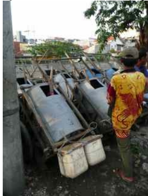
Figure 6.21: Manual collection of septage
