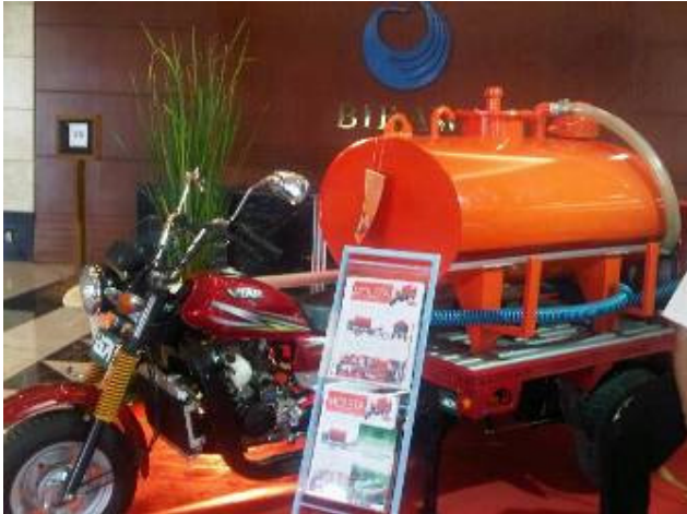
Figure 6.19: Motorized small-scale septage collection: vacuum motorcycle
