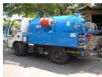
Photo by: Oni Hartono Date: October,29 '05 Location: Solo Remarks: (left) Balekambangan pond for flushing the sewerage system (centre) Tirtomoyo swimming pool for flushing the sewerage system (right) Truck Rom Combi, for maintaining the sewerage system
