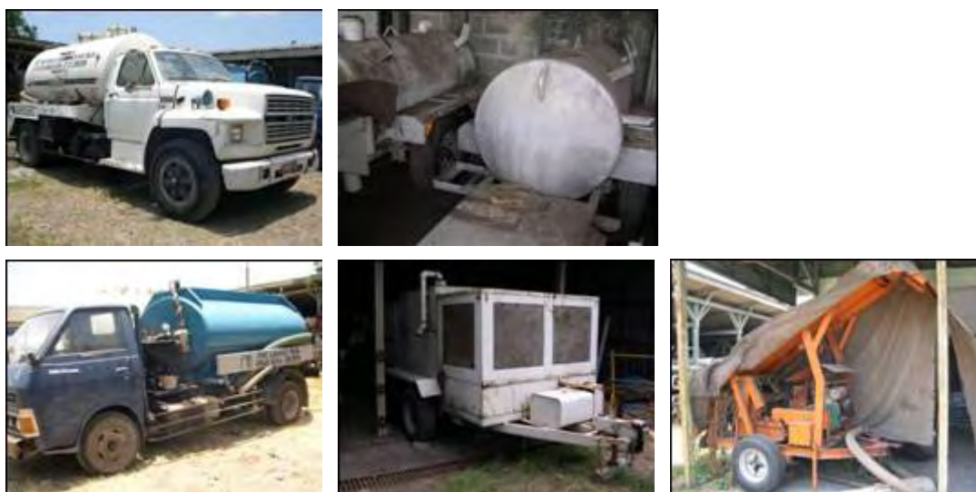
Photo by: Oni Hartono Date: October,06 '05 Location: PDAM Cirebon office (workshop) Remarks: Top (left to right): Sludge truck 'maxlife' 8 m 3 (bad condition) ; Sludge tank 'maxlife' 1 m 3 for small street (bad condition) Bottom (left to right): Sludge truck 'maxlife' 3 m 3 (good condition) ; jetting machine for flashing sewerage (bad condition) ; bucket machine for cleaning sewerage between manhole and manhole (good condition).
