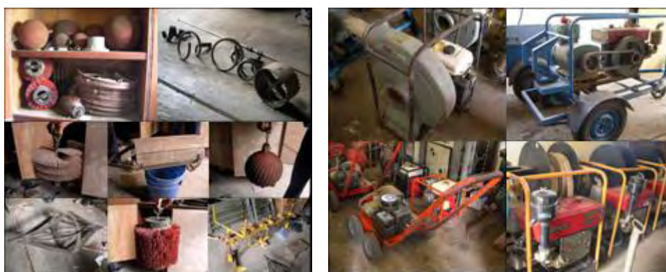
Photo by: Edzard Ruehe Date: October,10 '05 Location: Antapani office & workshop wastewater division (PDAM) - Bandung Remarks: (left): Equipment for sewer maintenance. (right): Equipment for maintenance sewer facility, from top left (rotate clockwise) Blower to bring gas out from sewer, Mobile genset for energy supply, Jetting for cleaning sewer with spray water, Rodding for cleaning sewer. All in good condition and still working.
