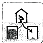
Figure 8-3: Future Twin Leaching Pit? (UNICEF/Spit, 2012)
