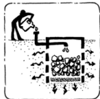
Figure 9-2: Gravel filled soakaway (Tilley, 2008)
