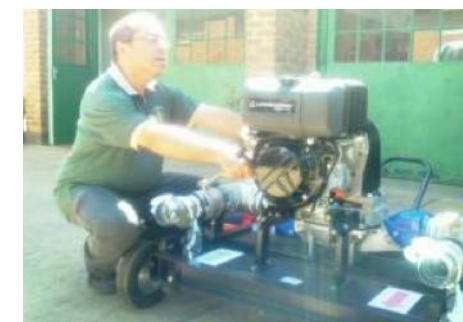
Figure 61: The sludge pump being serviced before use.
