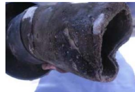
Figure 85: The active carbon cartridge has completely deteriorated.....but the plastic cover will only fit the cartridge.
