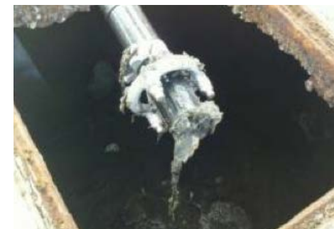
Figure 15: The 2" kit was blocked even with septic tank sludge as menstrual management materials are often flushed down the toilets.
