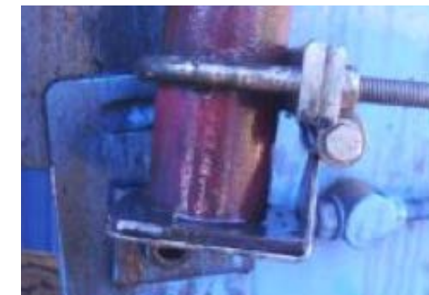
Figure 52: For the pressure chamber to be under vacuum the flap valve should be shut by lifting manually – it will remain sealed to maintain the vacuum.
