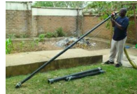
Figure 17: The 2" lance is far too long to be used in normal pit latrines.
