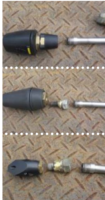
Figure 69: Deployment Karcher. The Karcher was checked to make sure that it was serviceable (lubricants for engine and pressure pump and fuel). Water supply should be ideally from the mains supply – but this is unlikely in emergency work, so we connect it to a filled drum.
