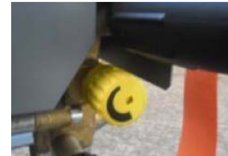
Figure 70: Details Karcher pressure washer. The pressure of the water jet is regulated by the knob.
