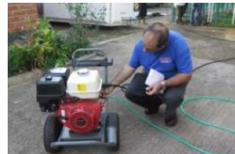
Figure 69: Deployment Karcher. The Karcher was checked to make sure that it was serviceable (lubricants for engine and pressure pump and fuel). Water supply should be ideally from the mains supply – but this is unlikely in emergency work, so we connect it to a filled drum.
