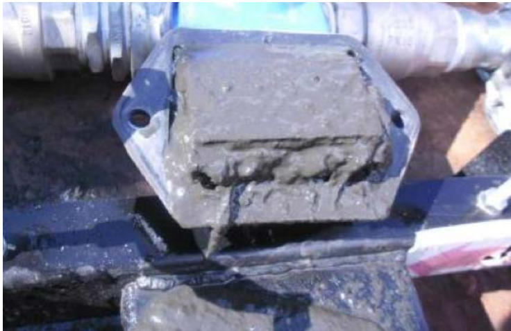
Figure 68: The delivery side port valve was also not sealing due to small pieces of cloth.
