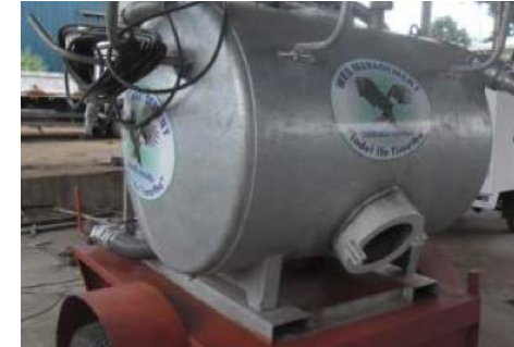
Figure 43: The inspection cover supplied by ROM was welded on by a local welding shop.
