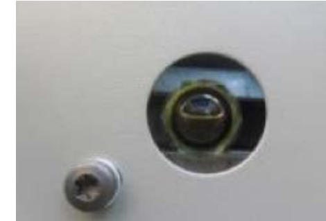
Figure 70: Details Karcher pressure washer. The pressure pump came already lubricated – inspection glass.
