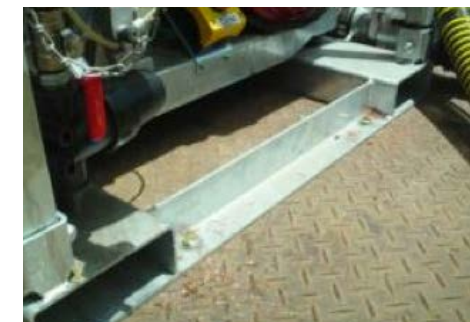
Figure 13: The ROM rig should be firmly bolted on its transport.
