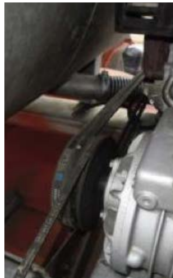
Figure 39: The drive belts broke and were replaced after 300 operations.
