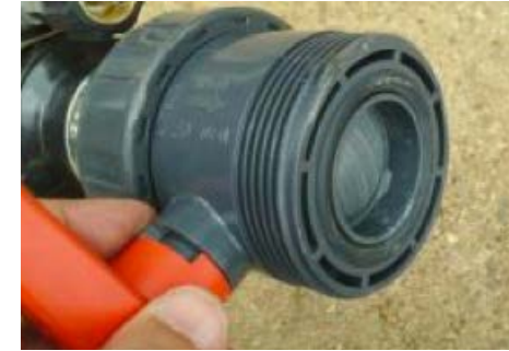
Figure 16: The plastic ball valve showed signs of abrasion after only a few operations and the threads were easily crossed by operators.
