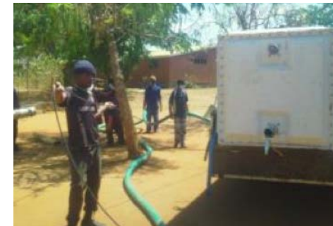
Figure 87: Due to the position of the discharge port, the tank cannot be wcompletely emptied of about 0.5 m 3 sludge.
