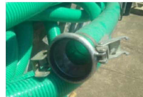
Figure 8: Camlock couplings should be of best quality in order to ensure efficiency of the machine and long service life.
