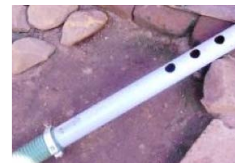
Figure 62: The suction lance has 25mm perforations to prevent large objects such as stones entering.
