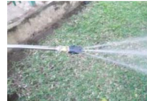
Figure 1: Spray pattern using a 4 jet nozzle at 100 bar.
