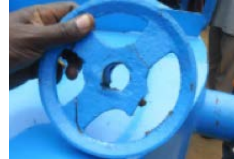
Figure 56: The original Vacutug pulley broke – and we failed a decent repair and could not find an off the shelf replacement.
