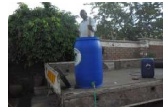
The water inlet to the pump was from a 200 lt drum, via 12mm plastic hose, with gravity feed (1 m). We eventually had to upgrade from 1/2" to 3/4" hosepipe to increase the output pressure from the nozzles.
