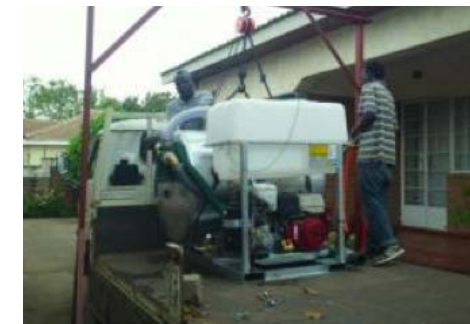
Figure 12: The ROM2 was easily deployed but required lifting gear.
