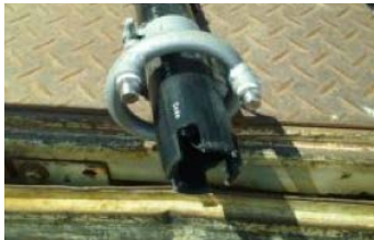
The standard Karcher nozzle fitted without problem to the lance (also Karcher)
