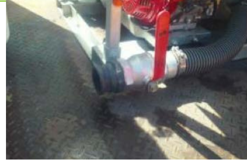
Figure 29: We fitted one of the plastic couplings.
