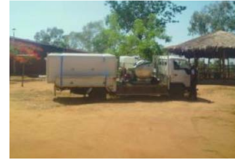
Figure 86: The tank was mounted on a 3 ton lorry, together with the ROM2. However it is advisable to mount the tank and possibly desludging pump in a 7 ton lorry.
