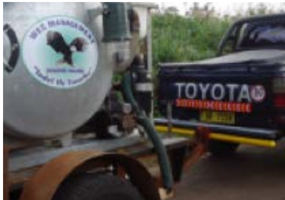
Figure 42: Trailer prototype using either 15" or 16" wheels for compatibility with towing vehicle. The trailer proved very stable on and off road. The 'bakkie' is also convenient for carrying 45m of 3" pipe (30m suction and 15 m delivery) plus equipment like safety clothes, buckets for rubbish, sprayer, fishing tools, etc.
