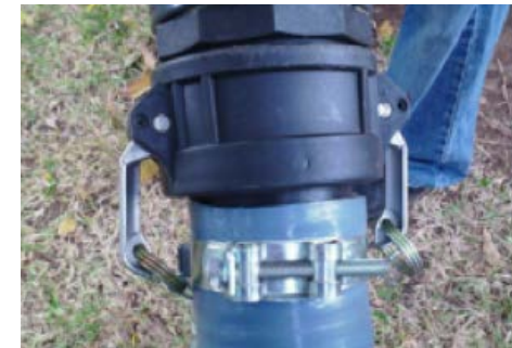
Figure 7: The coupling should be firmly anchored to the suction pipe using a high torque clamp band. Definitely don't use “jubilee clips”!
