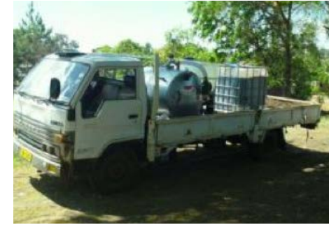
Figure 14: The 3 ton truck carrying 700 l 800 litres sludge in the ROM and 1000 litres sludge in the IBC for disposal at the Blantyre Sewage treatment plant. No spillages en route.
