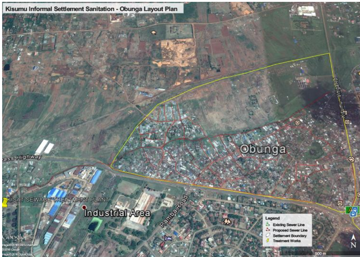
Figure 26: Obunga Sewer Lines
