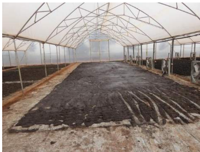
Figure 1: Solar drying in greenhouses of mechanically dewatered septage and faecal sludge to be sold as fuel to industries (Pivotworks, Kigali, 2016)
