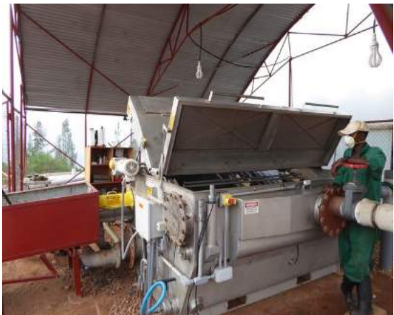
Figure 30: Sludge Belt Press by Pivotworks (Mechanical Dewatering)
