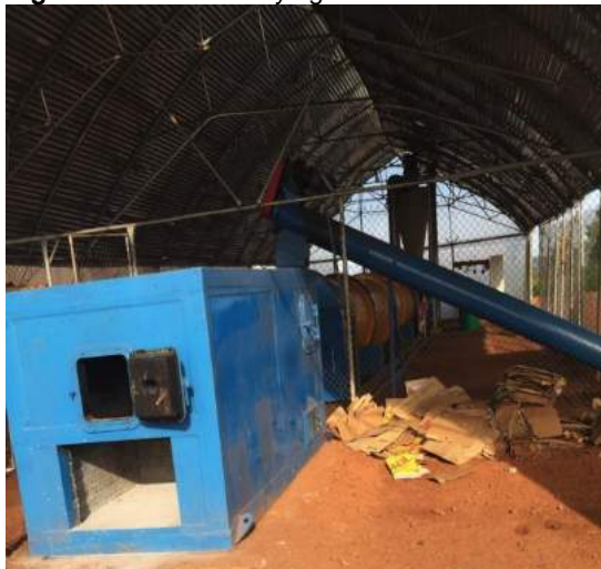
Figure 64: Thermal drying unit at Pivotworks, Kigali, 2016 (Photo: Henock Belete, 2016)
